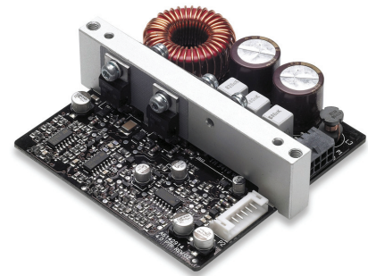
Figure 1: ICEpower500A Size: 9 x 9 x 2.7cm
